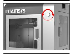
Use a leveling card and rotate the button until you feel a bit resistance.
