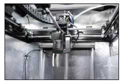
STEP 5: Open the front door to put the glass plate onto the platform. Align the three magnets on the glass plate to the magnet holders on the platform.
