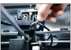
STEP 3: Disassemble the nozzle set cover, connect the motor connector to P7 on the pin board. and fix the cables with a cable tie.
