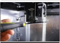
The leveling sensor is trigger ed
