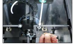
STEP 2: Install the motor on top of the extruder, and ensure the upper PEEK tube is securely inserted into its position.
