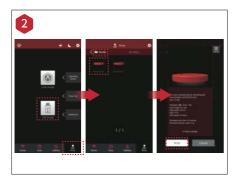
Open the "Print" tab, and choose "USB Storage" to open the file storage path. Select your dual extrusion file to check the printing parameters and settings. Press "Print" to start printing the test file.
