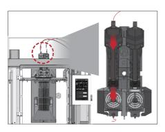
After loading both sides of extruders, press the "Utilities" tab on the bottom of the screen, and set the temperature of the left nozzle to match the requirements of the filament that you are using.
