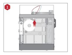
Locate the open end of the filament, and feed it through the guide tube. **NOTE:** The operation of the left extruder is the same as that of the right extruder. Here we take the left extruder as an example.
