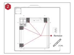
Peel off the yellow stickers and remove the 24 security spacers.
