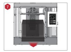
Open the front door, and remove the starter box and filament box from the printer's base.
