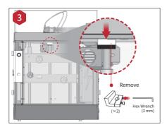
Select the largest of the included hex-head wrenches (3mm), and remove all four hex head security bolts from Z-axis clamps (2 bolts each).
