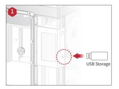
Insert the USB device that contains your sliced model files (.gcode or .data) into the USB slot on the side of the touchscreen
