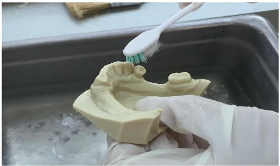
: Use soft brush to remove residual resin around undercut area and perform the second cleaning with IPA and ultrasonic cleaner. Be careful not to exceed 5 minutes in contact with the IPA and Model.
