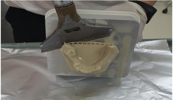
: Detach the printed Model from the build plate of the 3D Printer with tool like the picture above.
