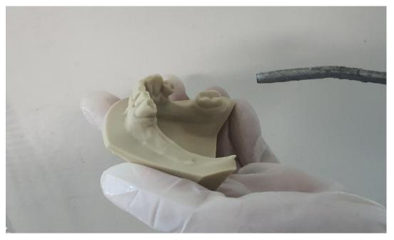
: Blow out the IPA using an air gun.
