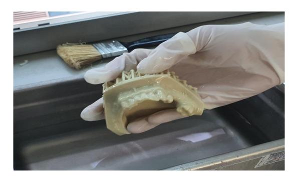
: Wash off the residual resin on the surface of the Model using IPA(alcohol 99%) and ultrasonic cleaner.
