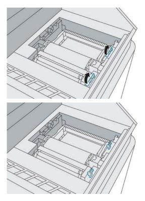
**9.** Rotate the handle until it is vertical, then pull it upwards to remove the cleaning roll module from the printer.
