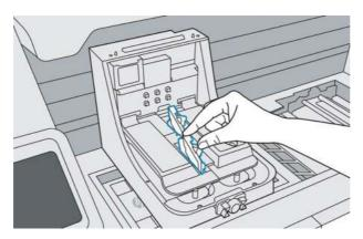
**24.** Put back the print carriage cover. Tighten the six screws.
