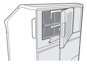
4. Insert the new filter. The arrows on it should be pointing towards the printer.
