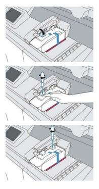
**10.** Pull the handle to unlock and rotate the lamp clockwise.
