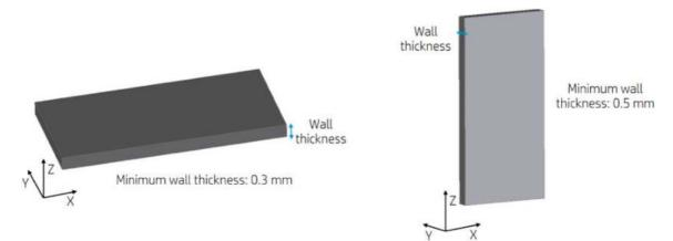
For color parts, in general, the minimum recommended **wall thickness** is 0.5 mm for short walls oriented in the XY plane, and 1 mm for short walls oriented in the Z plane.
