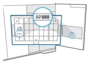
5. Put the alignment plate on the build platform and push it down as far as it will go. The HP logo on the plate should be facing up on the left of the build chamber.
