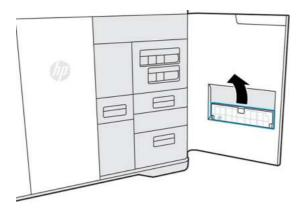
8. Ensure that the alignment plate AP number matches the number on the inside of the agent door. Close the door.
