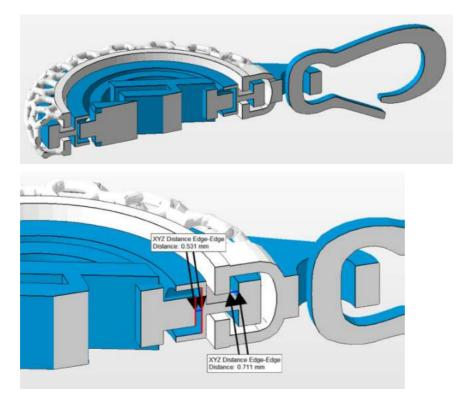
The inner circle with the HP logo will rotate freely after bead blasting although the clearance is quite low (less than 0.7 mm). This is because there is a small surface area of "contact" between the two surfaces that must freely move and an easy escape path for the unfused material to be removed during bead blasting.
