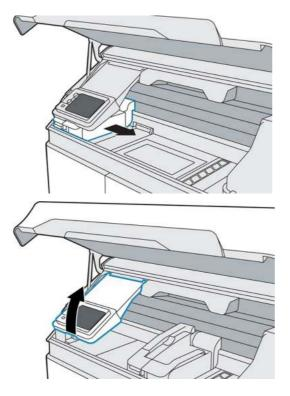
7. Vacuum all exposed surfaces, including the left wall and build-chamber filter cover.
