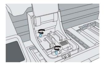
**16.** Carefully pull up the handle to remove the printhead, and place it on a flat surface with the nozzles facing up or to the side.
