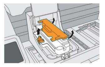
**21.** Orient and align the new printhead, then insert it into place, using the center post to guide the printhead. Ensure that all edges of the printhead lie flush with the carriage housing.
