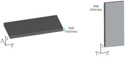
For parts with a high aspect ratio (>10:1), HP recommends increasing the wall thickness, or adding ribs or fillets to reinforce the part.
