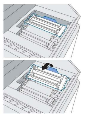
8. Disengage the two latches to release the cleaning roll module.
