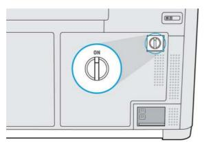
Leave the main power switch on at all times, unless you intend to move the printer.
