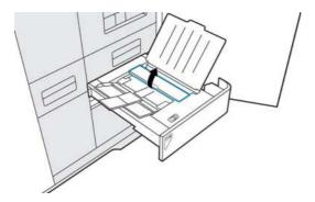
5. Locate the white plastic strip and the scanner glass strip. The glass strip is located underneath the scanner access bar on the base of the scanner, between the rollers and the white plastic strip.
