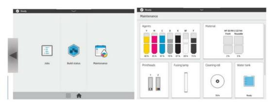
2. Check the Printhead Health Gauge for both Printhead 1 (Mono Printhead) and Printhead 2 (Color Printhead):
