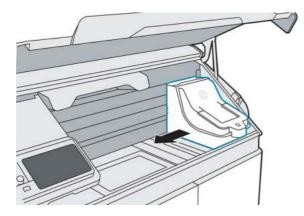
2. Remove the printhead cap.
