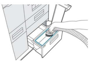
6. Vacuum any material from the bottom of the air exhaust filter.
