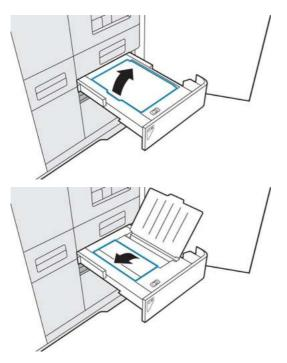
4. Rotate open the scanner access bar by reaching under the center tab and pulling up on the textured surface underneath.
