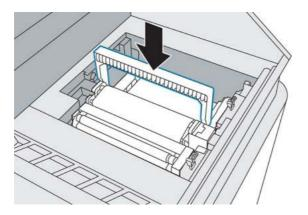
14. Engage the two latches to secure the cleaning roll module.
