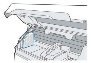
6. Disengage the latch on top of the filter.
