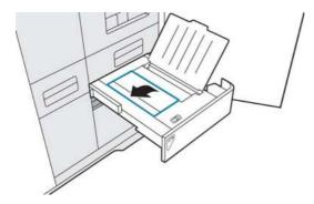
**17.** Load the first alignment page face-down on the scanner input tray.
