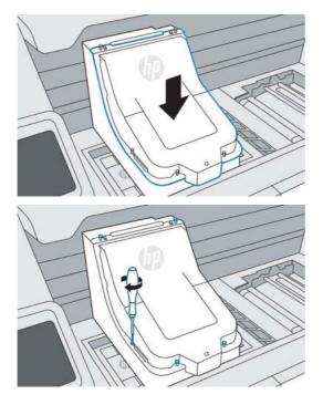
25. Tap Finish & Check. Leave the print carriage centered. Close the top cover and tap Continue on the front panel; when the priming tray is detected, tap Prime. Priming will take about 20 minutes.
