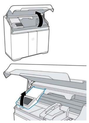
2. Pull the fusing carriage from the left of the build chamber to the center.
