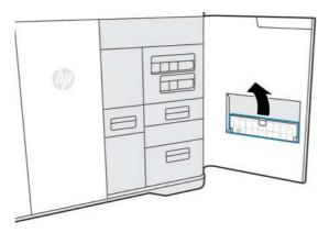
Each printer has one alignment plate. The number on the plate should match the number on the door.
