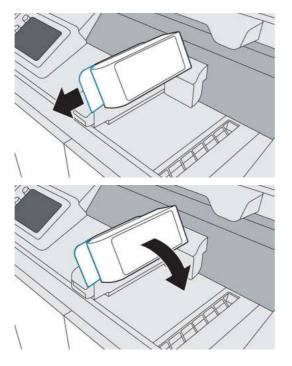
9. Push the lamp release handle back into place to connect the lamp module to the printer.
