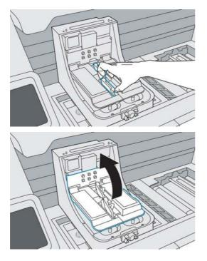
**15.** Loosen the two thumb screws at each end of the printhead until the printhead is released.
