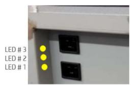
If the printer fails to power on, and the front panel is blank, call your support representative and describe the status of these three LEDs.
