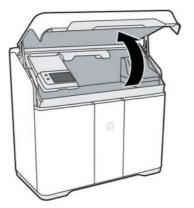
4. Open the agent door, and take the alignment plate from inside the door.
