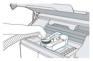
4. Pull the lamp release handle to disengage the lamp module from the printer.
