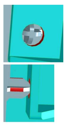
• **Minimum spacing and clearance** between parts printed as assemblies. Assembly parts that are printed together should have a minimum clearance of 0.7 mm. Parts with thick walls or large surface areas where the assembled features will fit together should have a larger gap to ensure sufficient material escape paths.
