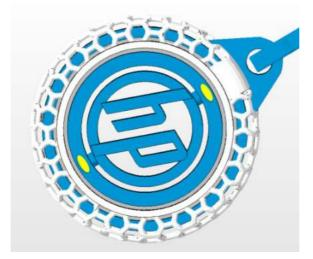
• Hollow closed geometries. Multi Jet Fusion is a process in which the parts are built by selectively fusing the desired areas of a material-based layer. If the parts printed are hollow, the unfused material can either be trapped inside the fused walls of the part or drain holes need to be added to the design to remove the material. The minimum recommended diameter of the holes is 5 mm; preferably larger, for ease of cleaning. HP recommends including at least two holes.
