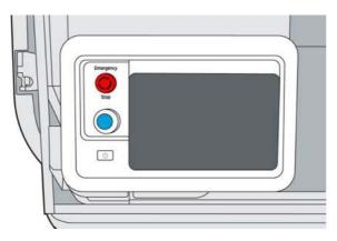
6. Wait for the front panel to indicate that the printer is ready. This can take several minutes. When initialization is complete, the front panel displays a ready message. If a system error message is displayed, see <u>System errors on page 155</u>.
