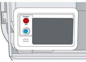
To turn off the printer for an extended period of time, first turn it off with the obstruction; wait for it to shut down completely; then turn off the main switch at the rear of the printer.
