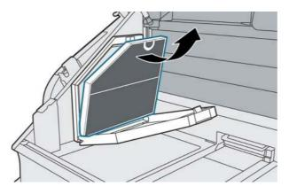
8. Insert the new filter, ensuring that the blue line on the filter is facing the interior of the print area.
