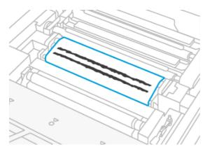
If there is only one mark, tap **One mark** on the front panel; the cleaning roll may have been inserted incorrectly. Try reinserting the cleaning roll module, and ensure that the latches are fully engaged.
