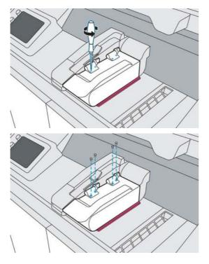
6. Pull the lamp release handle, lift the module, then remove it from the printer. Used lamps can be recycled through HP's Planet Partners Program, where available. Visit <u>http://www.hp.com/recycle/</u> for more information. Where the program is not available, dispose of the lamp according to local regulations.
