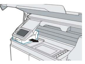
**3.** Inspect the top and sides of the fusing carriage. If you see any material there, use an explosion-protected vacuum cleaner to remove it.
