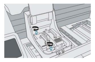
23. Pull down the printhead cover over the printhead, and secure both clips.
