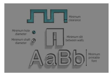
• **Engraving.** Multi Jet Fusion technology allows you to print letters and drawings with a very high resolution and definition.
