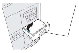
4. Add distilled or deionized water to the tank until it reaches the full line.
