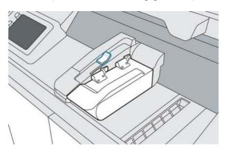
5. Lift the lamp handle and rotate the lamp to the left, then push to lock it into the cleaning position.
