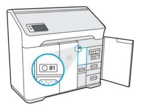
2. Check that the wayfinding LED is on, next to the access door to the material reclamation filter. Open the material reclamation filter by pushing the top left corner.
