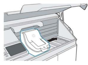
6. Move the fusing carriage to the right and lift up the front panel.
